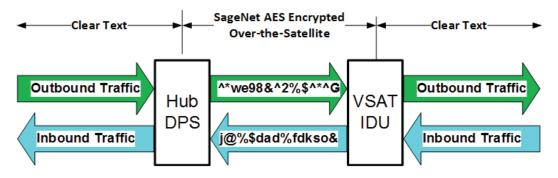
When a remote VSAT terminal is configured to operate in a secure mode, all customer data traffic that is transmitted over-the-satellite interface is encrypted. Following the VSAT network Layer-2 Link-Connect process, the remote VSAT initiates a procedure to exchange with the hub DPS module all the necessary parameters to secure Layer-3 communications (this group of parameters is called "SA" or Security Association). The following actions occur during this process:
