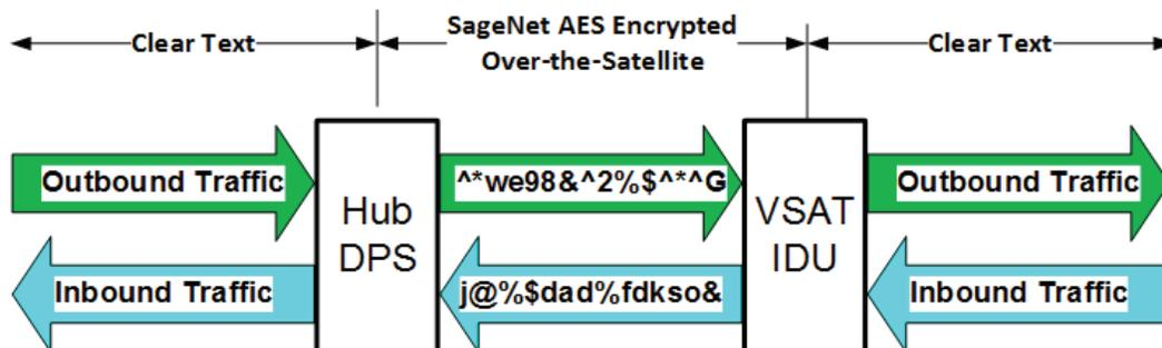
When a remote VSAT terminal is configured to operate in a secure mode, all customer data traffic that is transmitted over-the-satellite interface is encrypted. Following the VSAT network Layer-2 Link-Connect process, the remote VSAT initiates a procedure to exchange with the hub DPS module all the necessary parameters to secure Layer-3 communications (this group of parameters is called "SA" or Security Association). The following actions occur during this process:
